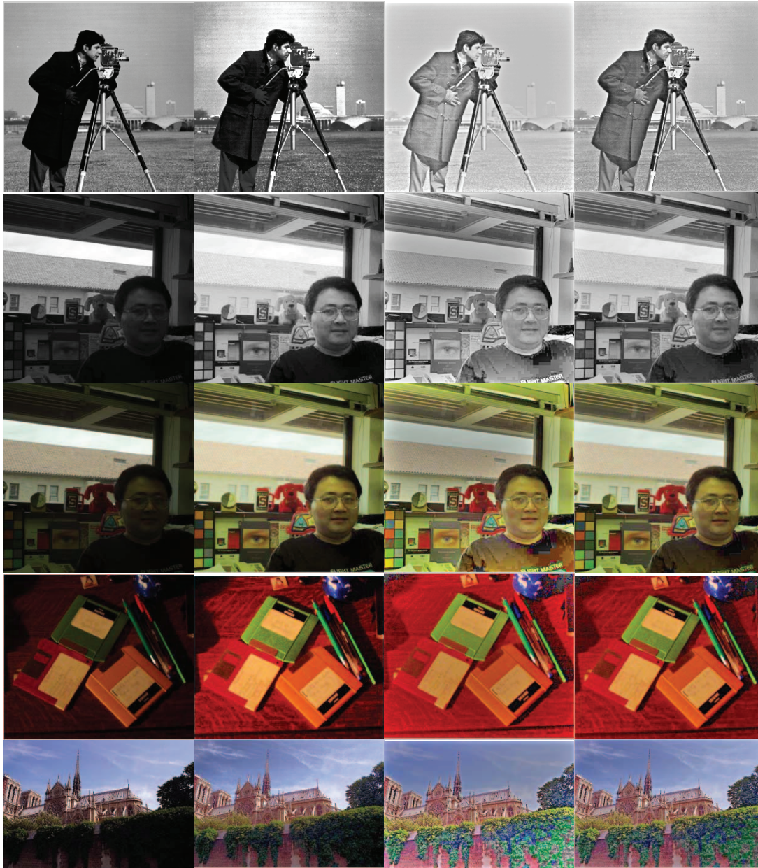
Figure 4. Fusion Results of MSR result and histogram equalization result: (a) Origin Images (b) Histogram equalization result (c) MSR result (d) Fusion result of MSR and histogram equalization.
