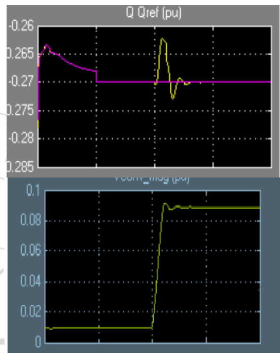
Figure 6: Waveforms of Voltage and Reactive power for UPFC
