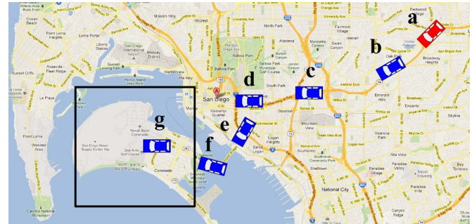
Fig. 9. Geographic location-based security mechanism. The shaded square is the naval base. Only the vehicles in the shaded rectangle region (i.e., vehicle g can decrypt and access the received ciphertext sent by vehicle a ).
