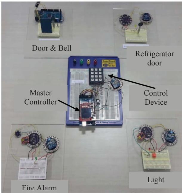
Figure 3: Prototype System Setup
